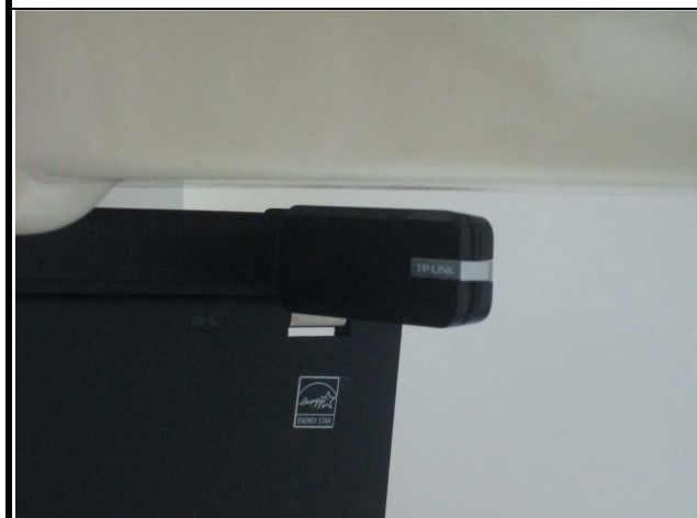
Test Position 3: USB Vertical Front with 0.5 cm Gap
