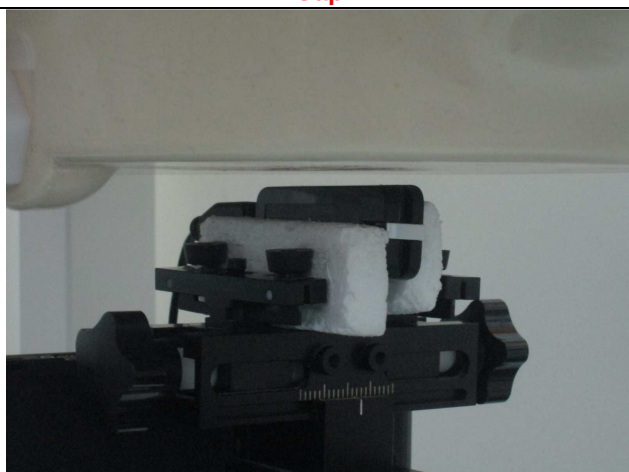
Test Position 4: USB Vertical Back with 0.5 cm Gap
