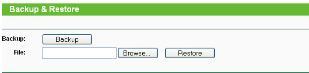
Figure 4-36 Save or Restore the Configuration
