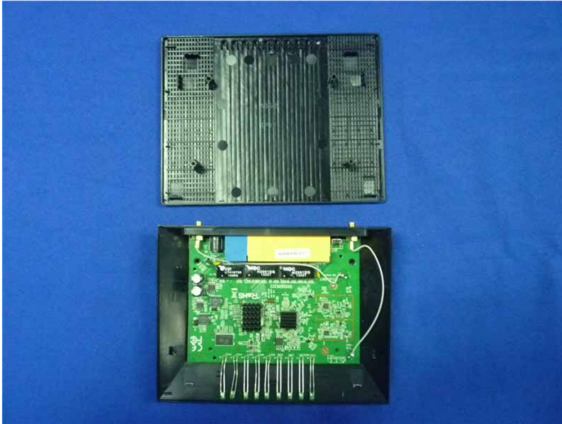
Figure 9 Inside of the EUT
