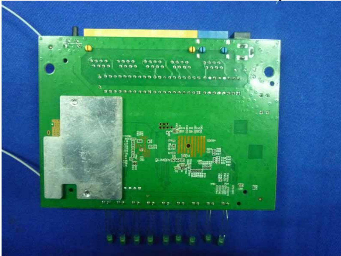
Figure 13 Components Side of the PCB
