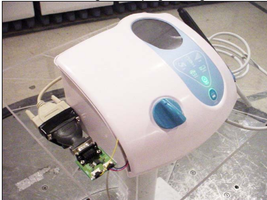
Front view of the EUT showing the test programming fixture on the left side.
