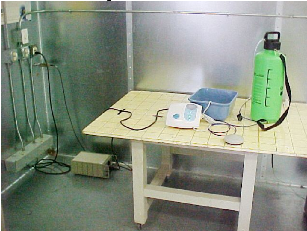
View of the EUT during the conducted emissions onto AC mains.
