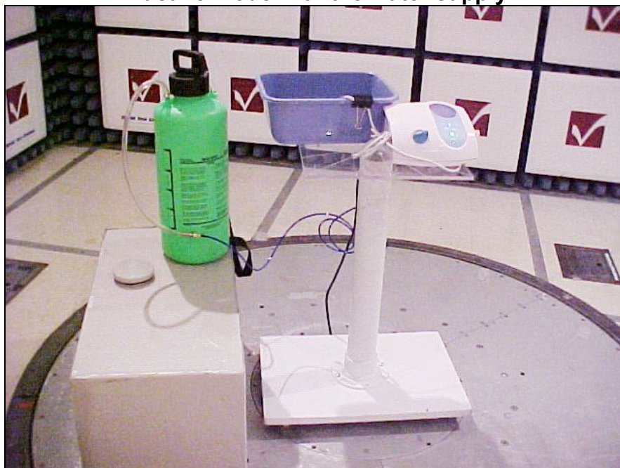
View of the EUT showing the setup on a pedestal during radiated emissions testing In active mode with the water supply.
