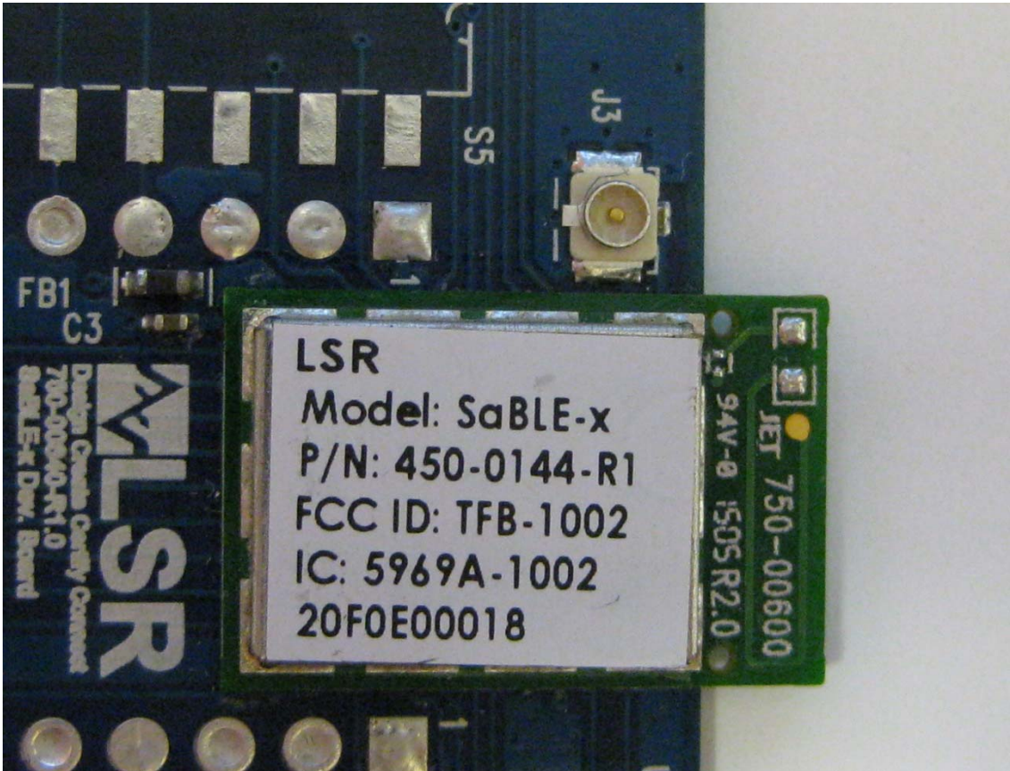
Module with u.fl connector
