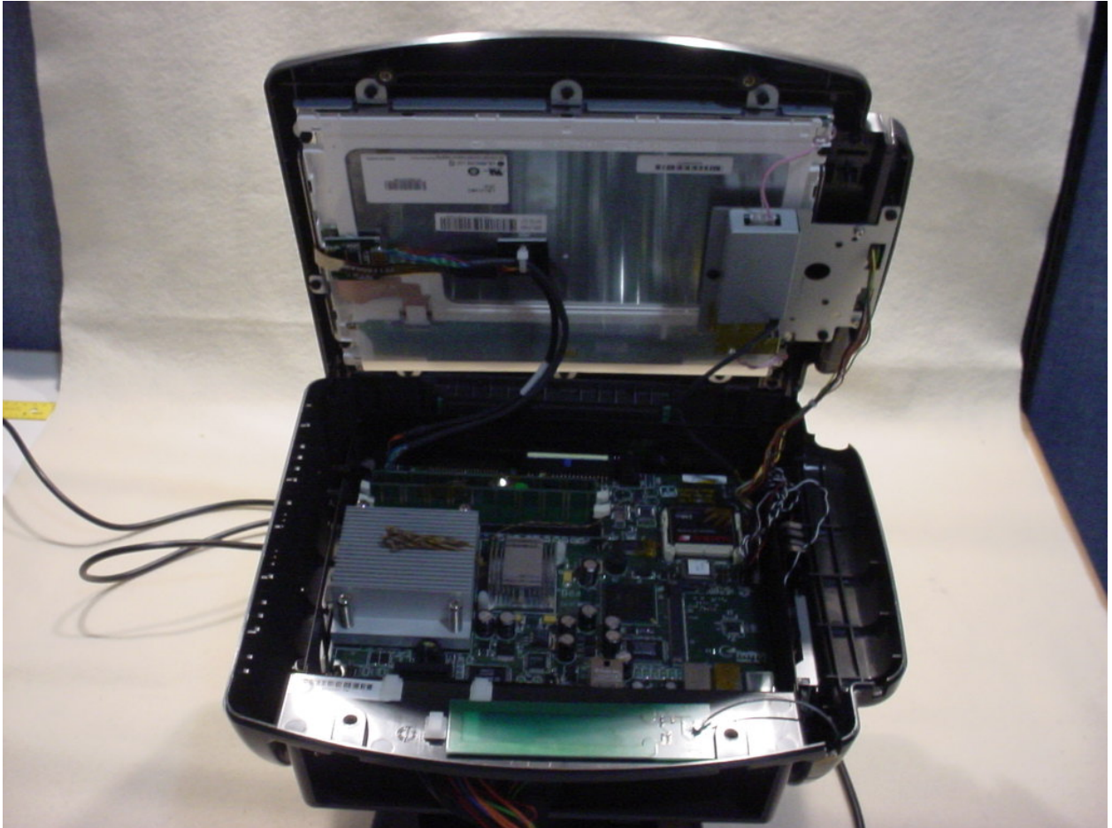
Figure 1: Inside View Showing Motherboard, Display Board and Antenna
