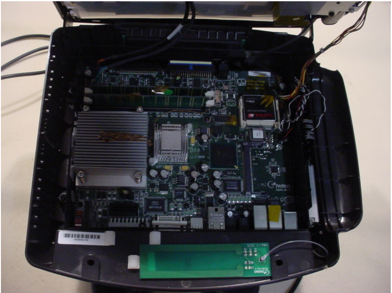
Figure 2: Inside View Showing Motherboard and Antenna
