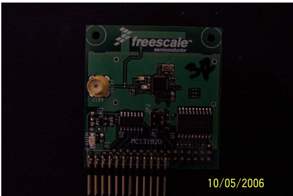
Top of EUT (Shield removed)
