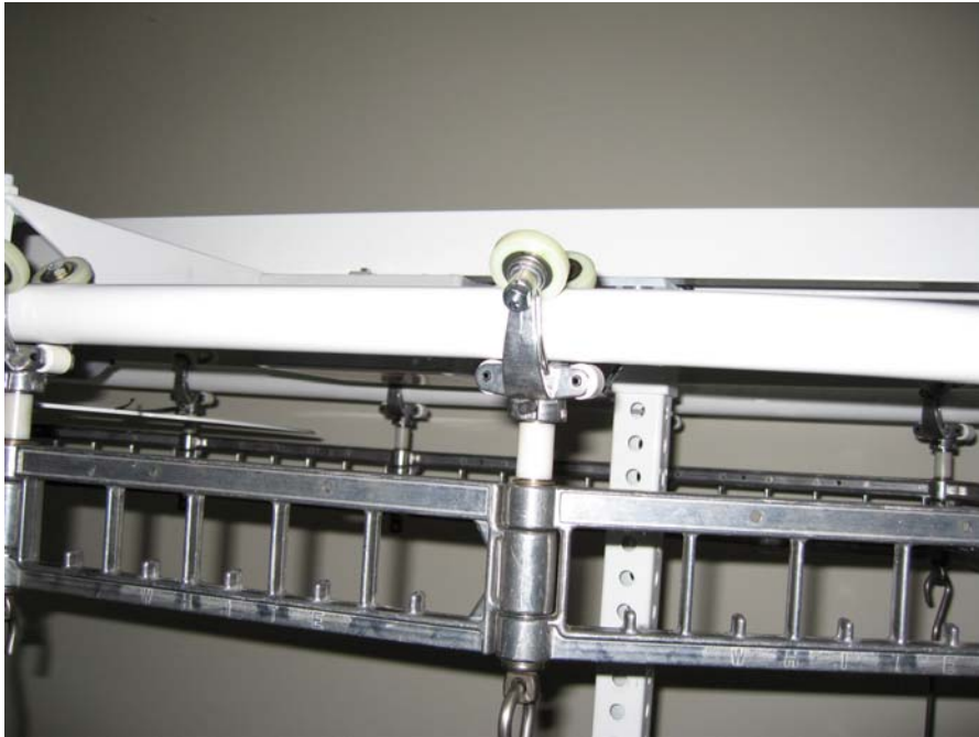
Example: View of the wheel and chain assembly on the conveyor.
