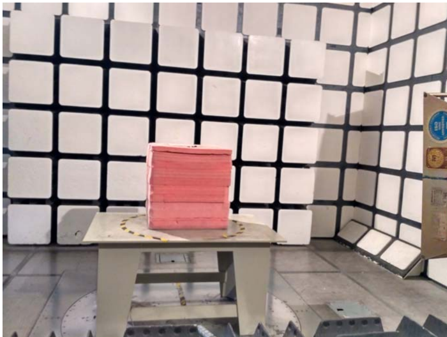
Radiated Emissions View (Above 1 GHz)
