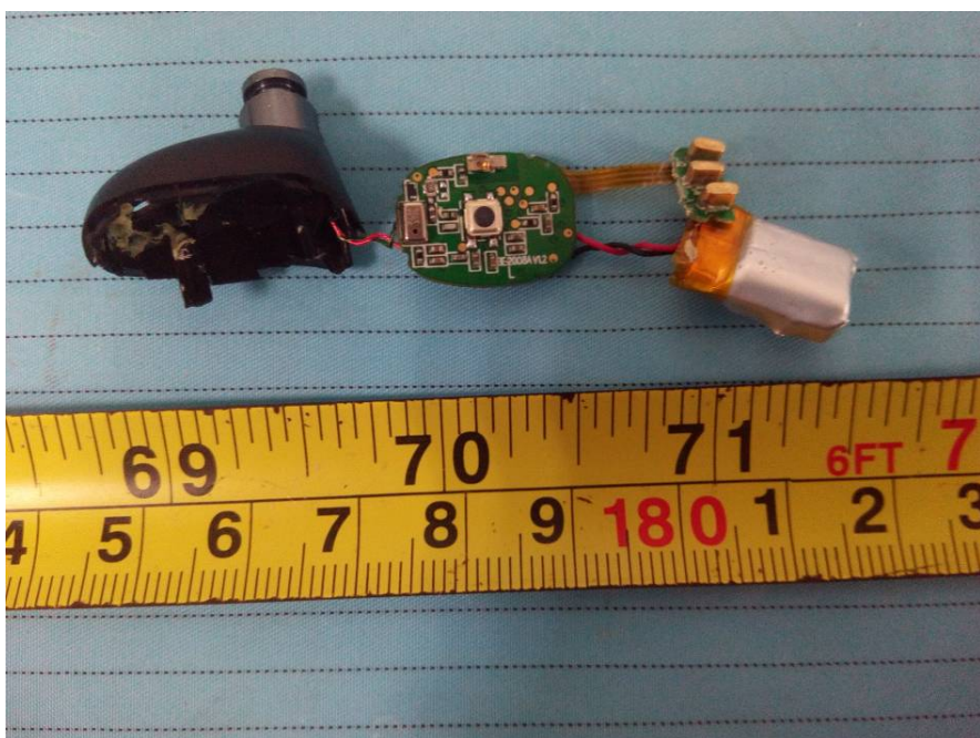
EUT – Main Board Top View (Earbud)
