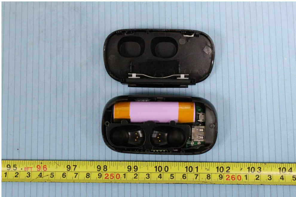
EUT – Cover off View 1 (Portable Charging Case)
