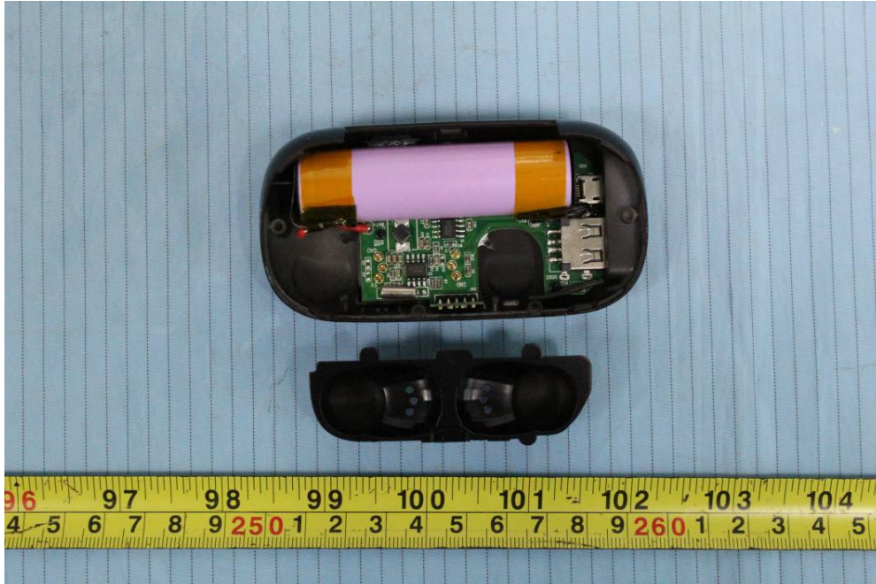
EUT – Cover off View 2 (Portable Charging Case)
