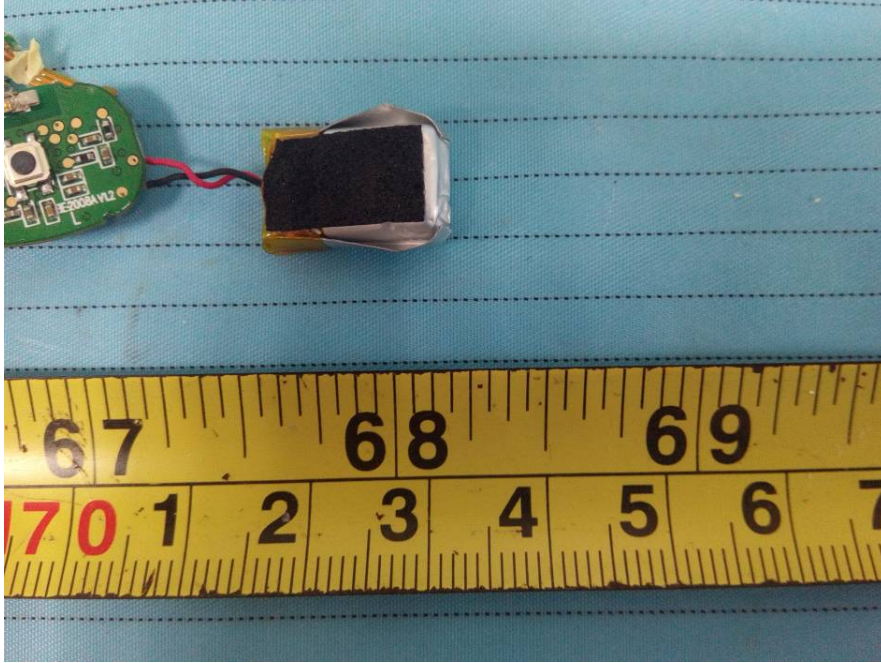
EUT – Battery Top View 1 (Earbud)
