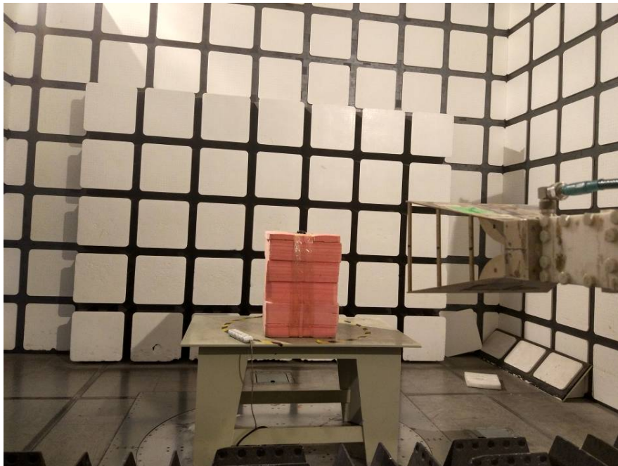
Radiated Emissions- Side View (Above 1 GHz)
