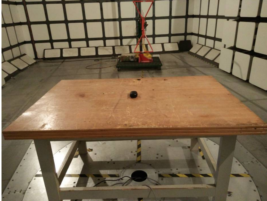
Radiated Emissions-Side View (Below 1 GHz)
