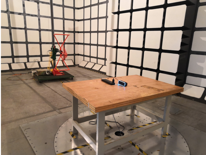
Radiated Emissions View (Below 1 GHz)
