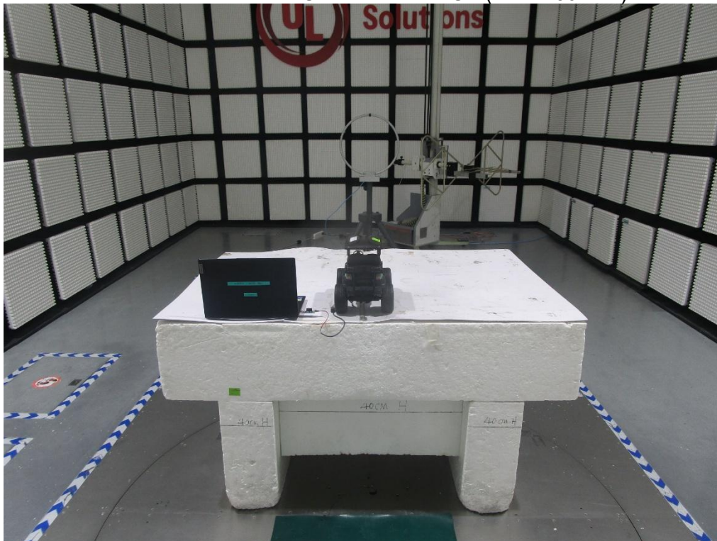
RADIATED RF MEASUREMENT SETUP (Below 30MHz)
