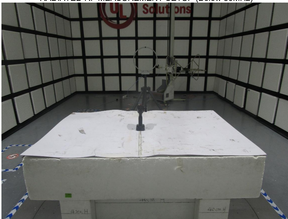
RADIATED RF MEASUREMENT SETUP (Below 30MHz)
