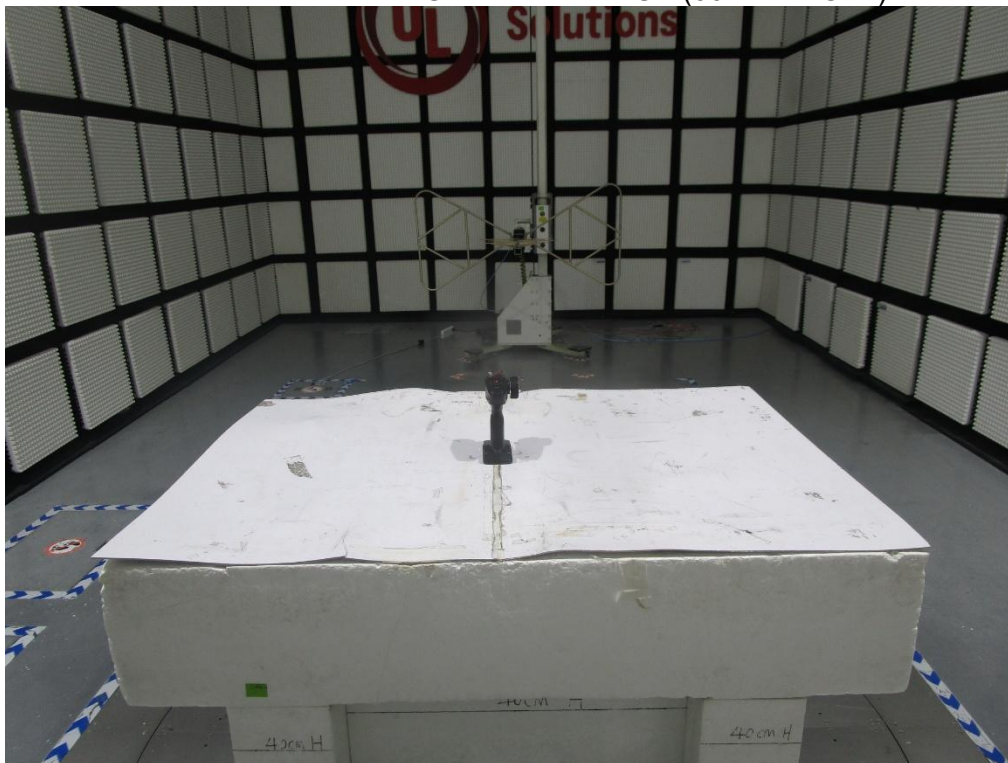
RADIATED RF MEASUREMENT SETUP (Below 30MHz)
