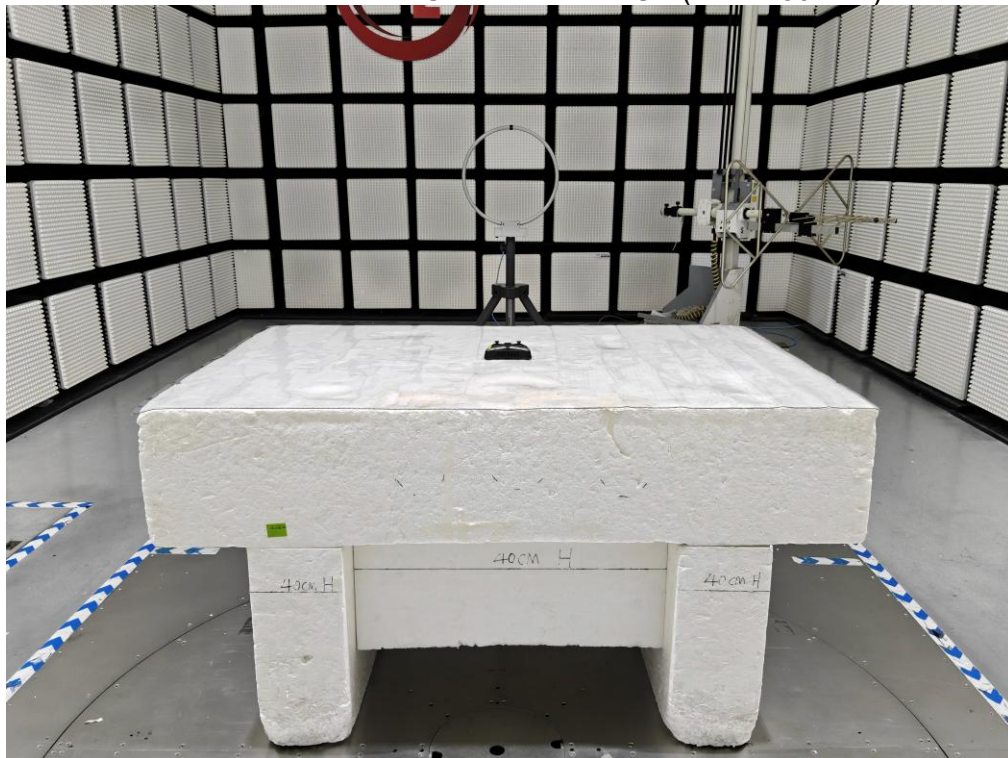
RADIATED RF MEASUREMENT SETUP (Below 30MHz)
