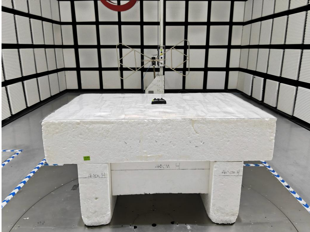
RADIATED RF MEASUREMENT SETUP (30MHz~1GHz)
