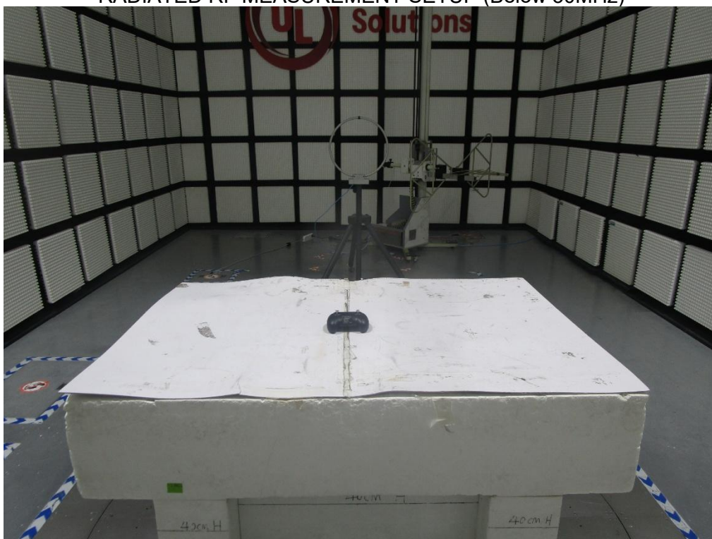
RADIATED RF MEASUREMENT SETUP (Below 30MHz)
