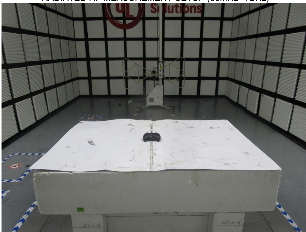
RADIATED RF MEASUREMENT SETUP (Below 30MHz)
