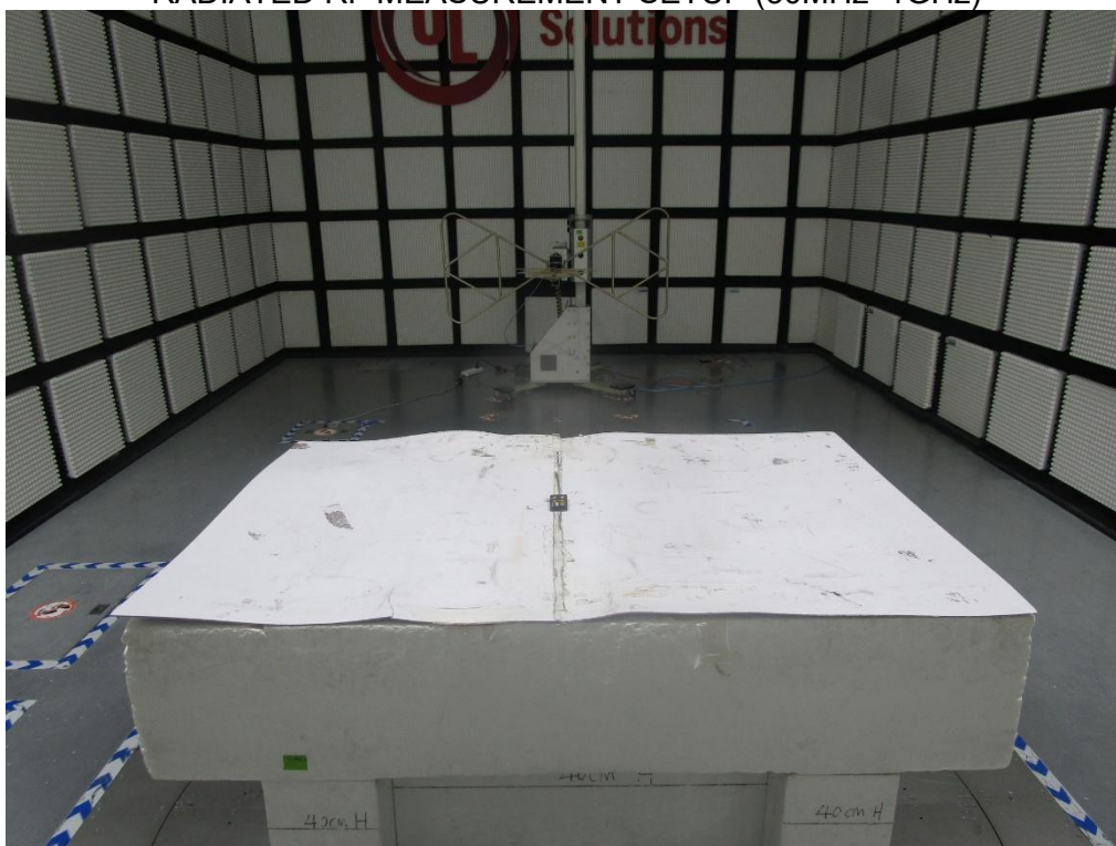
RADIATED RF MEASUREMENT SETUP (Below 30MHz)
