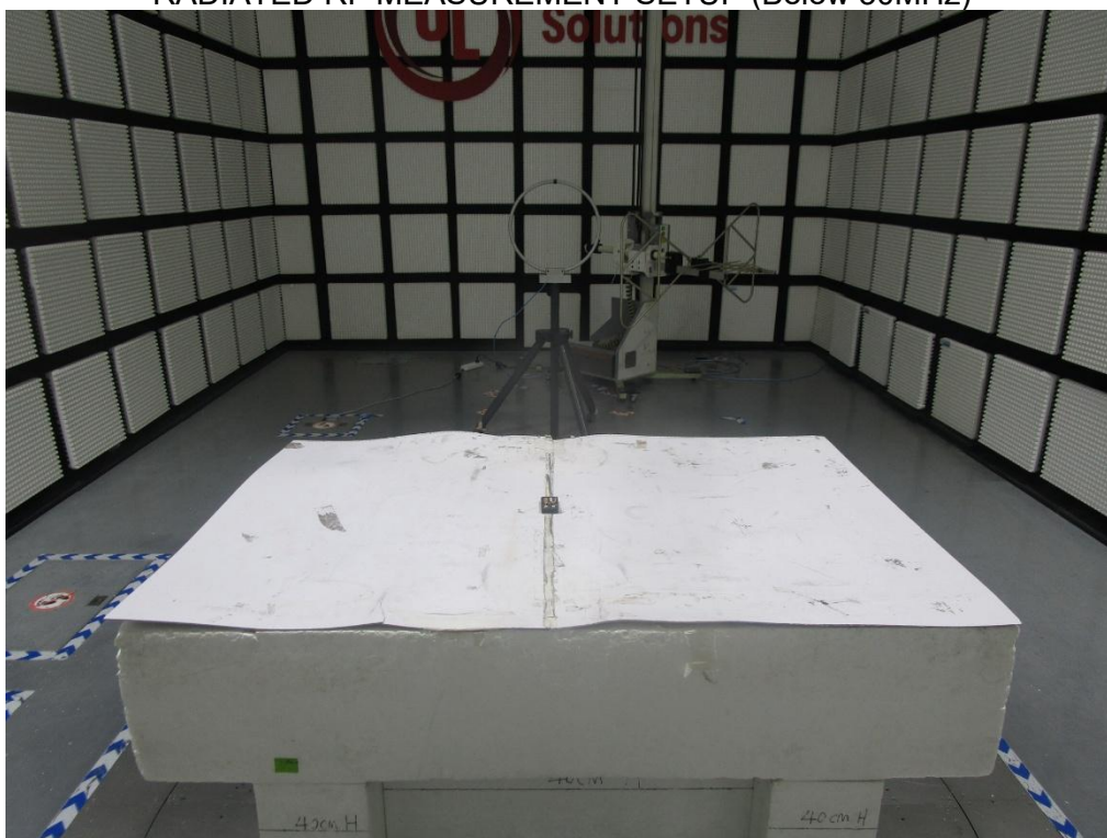
RADIATED RF MEASUREMENT SETUP (Below 30MHz)
