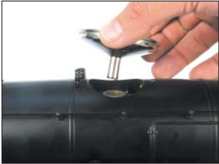
fig. #11 Metal funnel placed in locomotive
