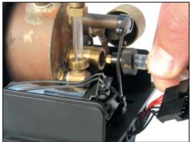
fig. #14a Connecting butane hose into the locomotive boiler
