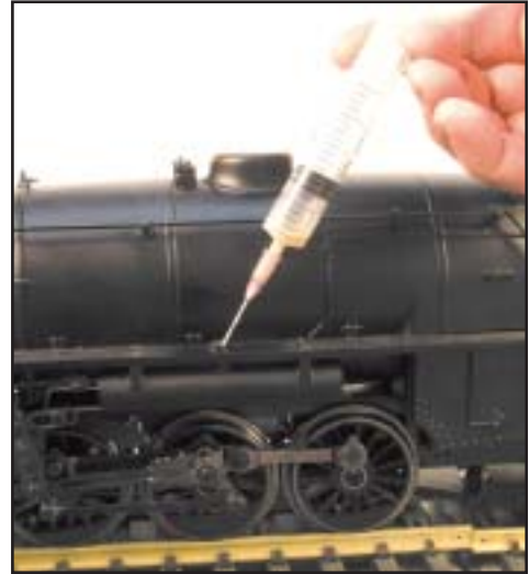
fig. #9 Inserting the oil with a syringe
