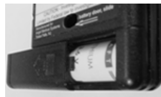
Fig. 11a – d. Replacing the Battery
