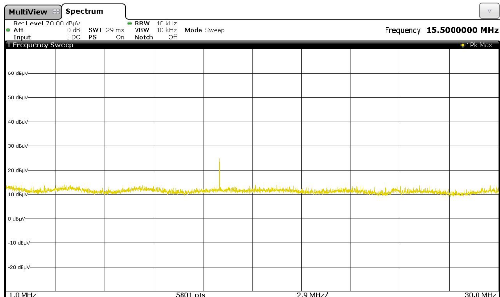
172414_112.png: Spurious emissions from 1 MHz to 30 MHz
