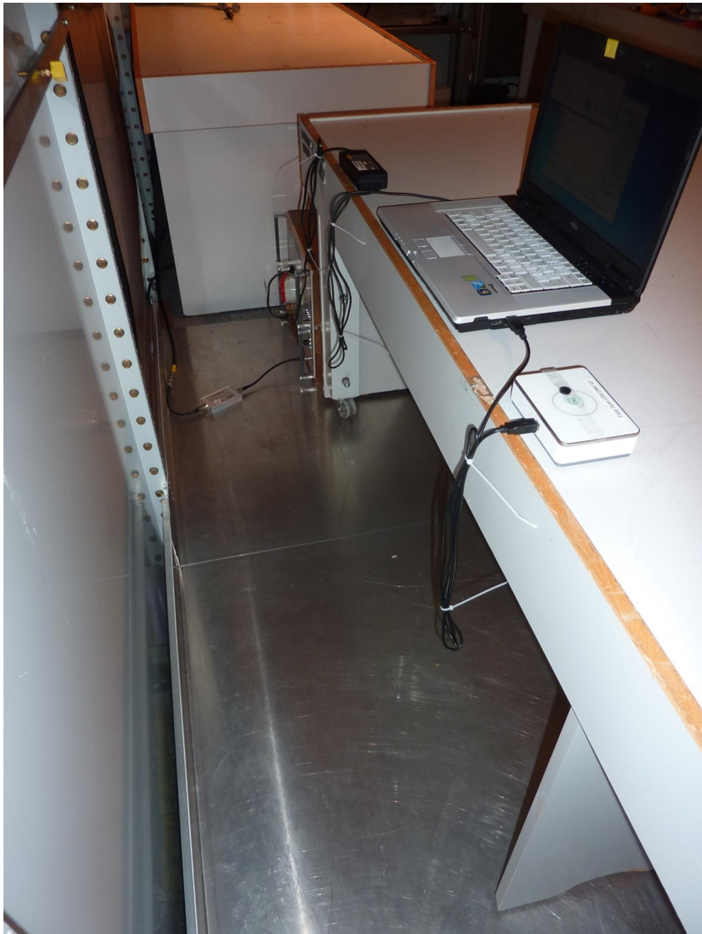
172414_26.jpg: EasyScan USB, test set-up shielded chamber
