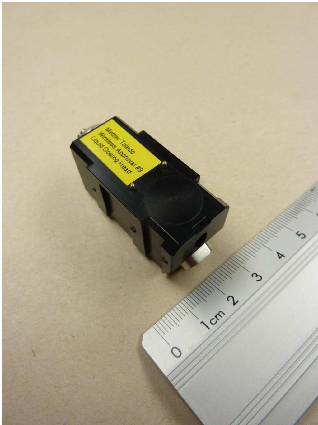
161006_10.jpg: Liquid dosing head (with TAG), 3D-view 1
