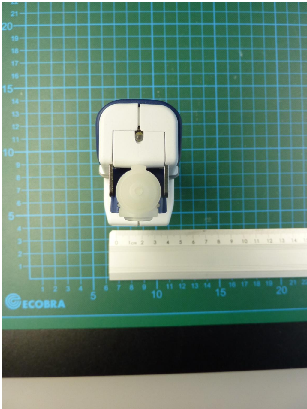
161007_3.jpg: Quantos HPD with powder dosing head, bottom view
