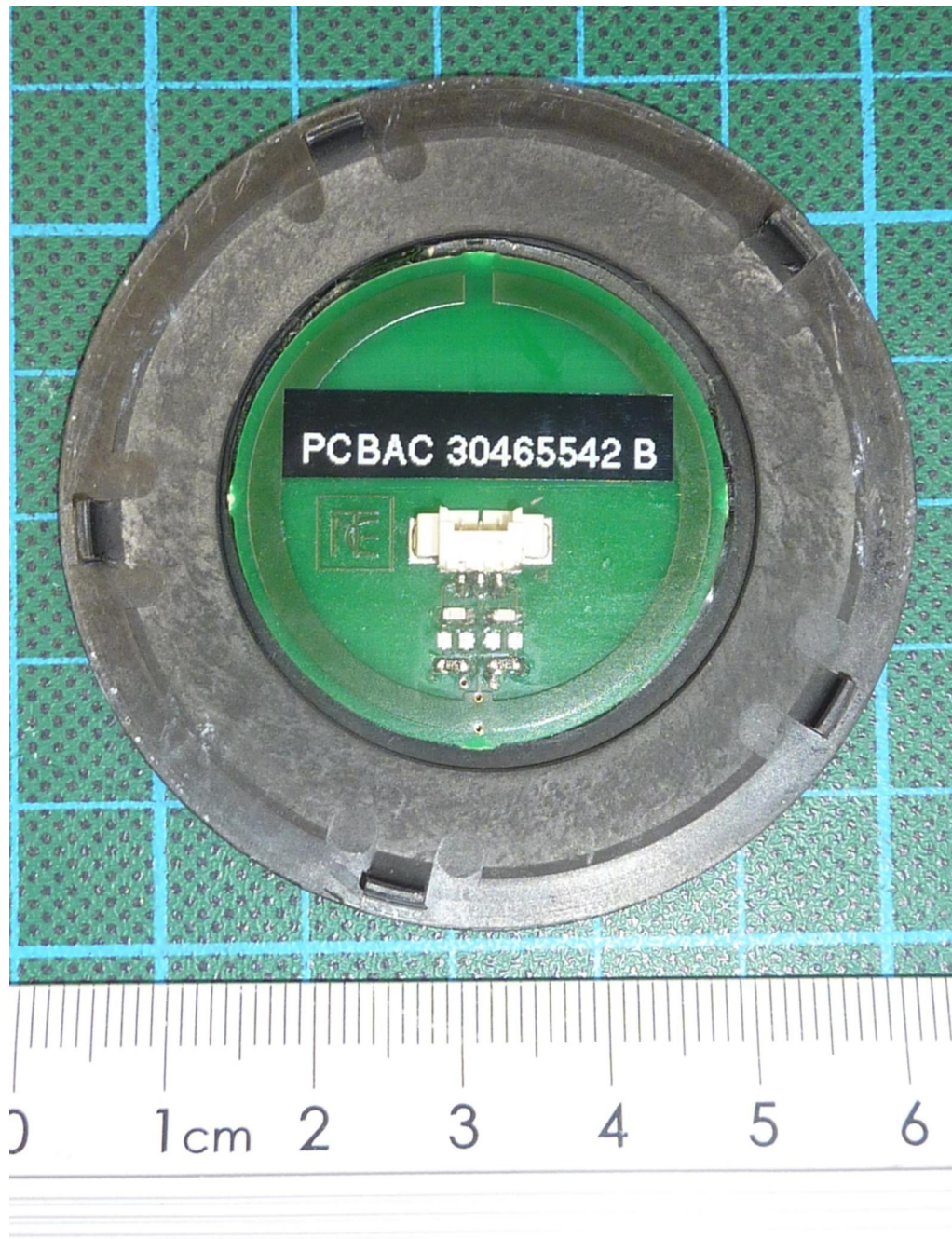
172416_o.jpg: SmartScan, antenna PCB
