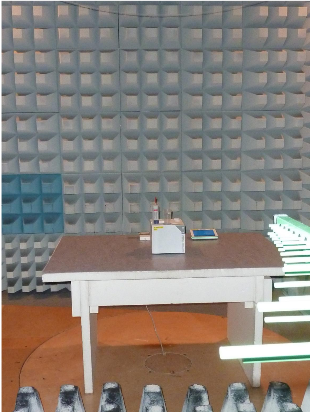
161791emiB3.jpg: EUT (Excellence Titrator T9), test setup fully anechoic chamber
