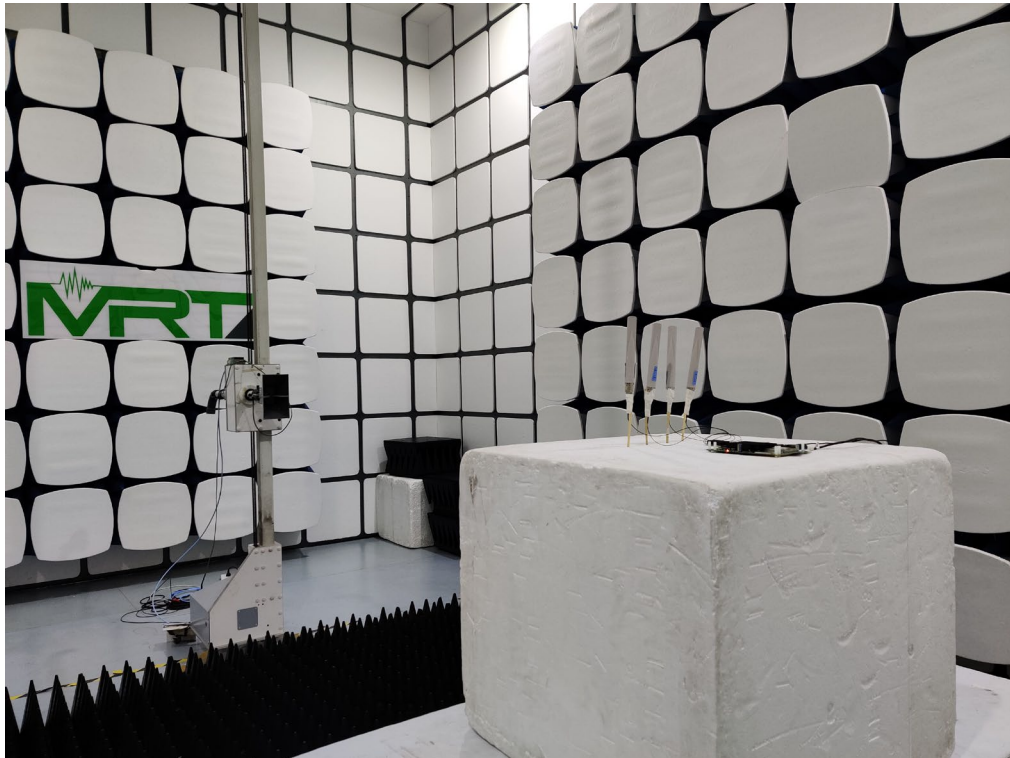
Description: Radiated Spurious Emissions Test Setup (above 1GHz) - Antenna 5#
