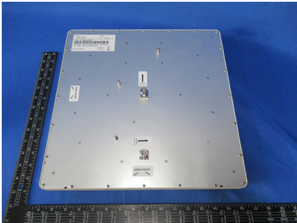
(6) EUT Photo (Panel Antenna 22.5dBi)
