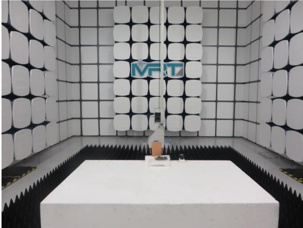
Description: Radiated Emission Test Setup for 18GHz ~ 40GHz (Panel Antenna 1#)
