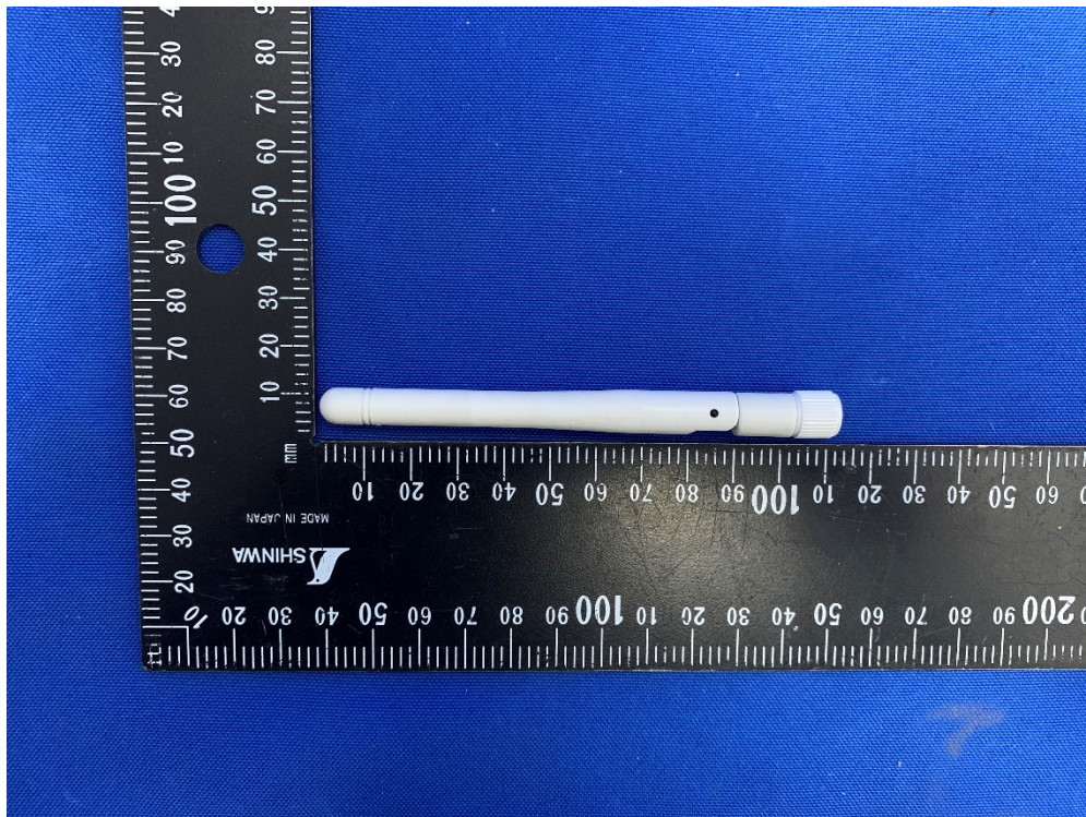
(9) EUT Photo - Omni antenna 2#
