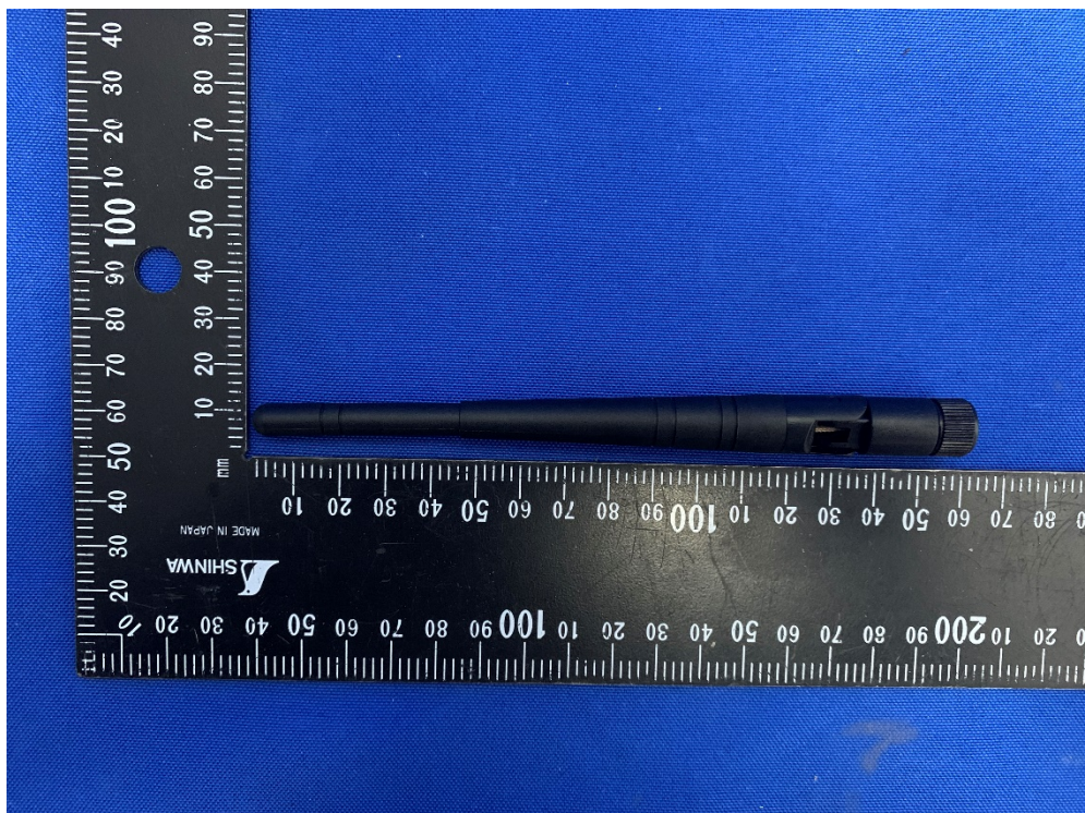
(10) EUT Photo - Omni antenna 3#
