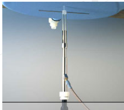
Photograph of the dipole Antenna
