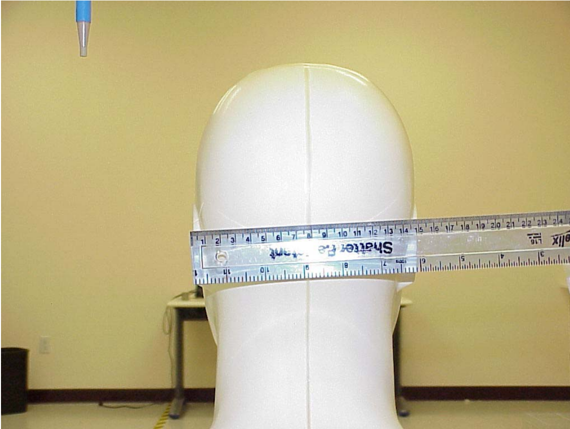
Photo 9. Photo to demonstrate 15 cm Z-axis head phantom
