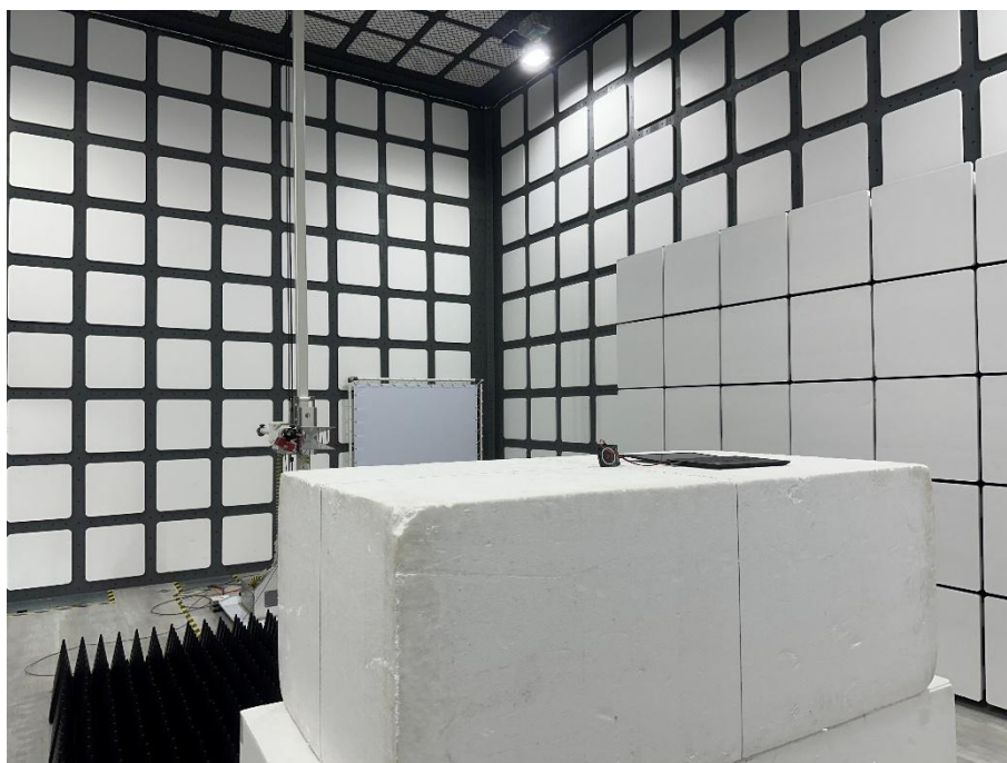
Set-up for Spurious Emissions Rear View
