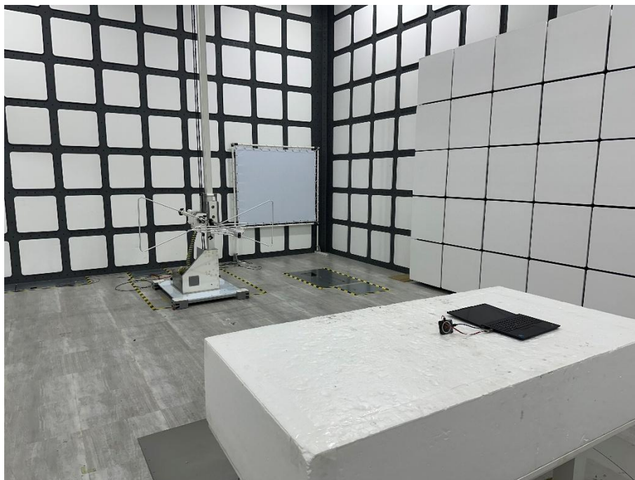
Set-up for Spurious Emissions Rear View
