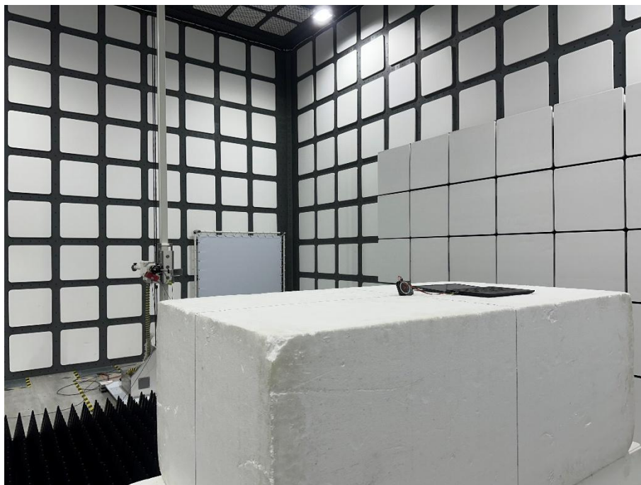
Set-up for Spurious Emissions Rear View
