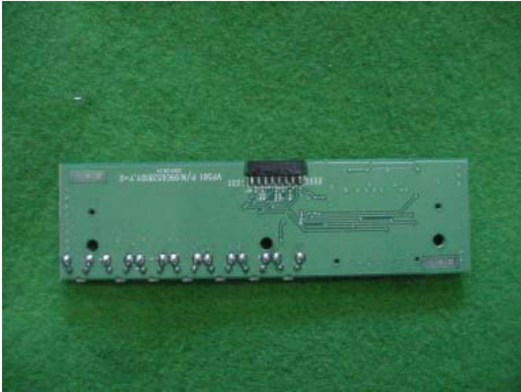
Rear Side of Controller Board
