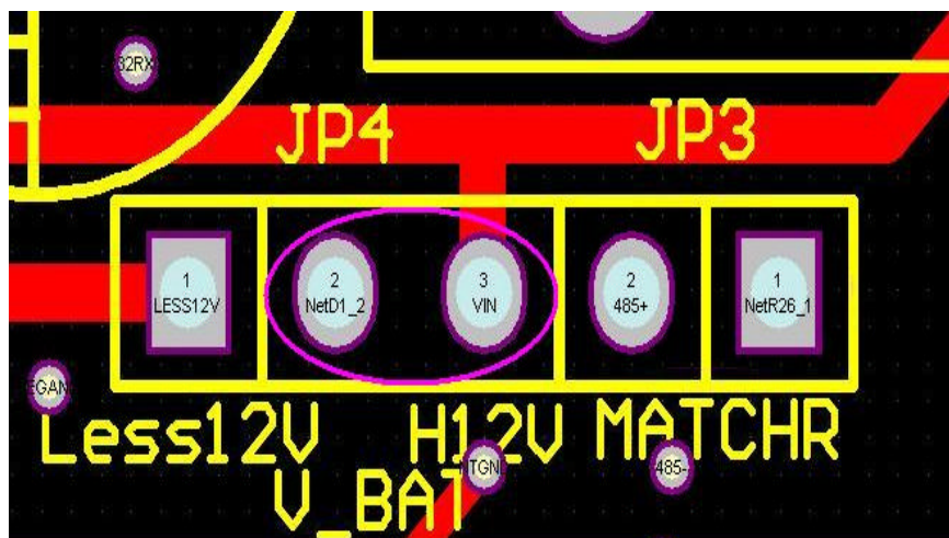
Figure 2.5 Power Supply 48V>Vin>12V
