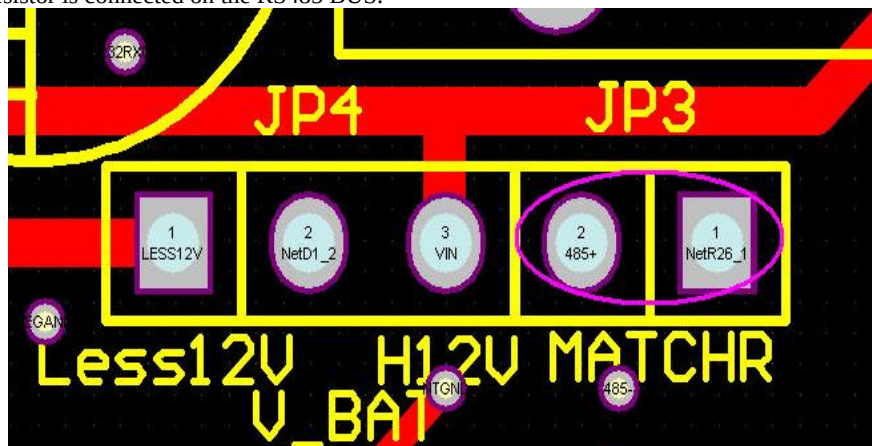
Figure 2.3 RS485 Terminal Resistor Is connected
