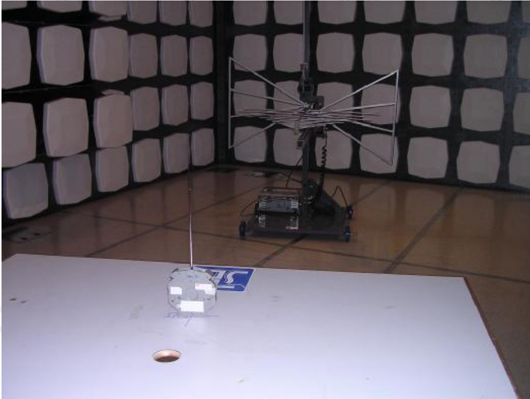
Measurement of Radiated Emission Test Set Up
