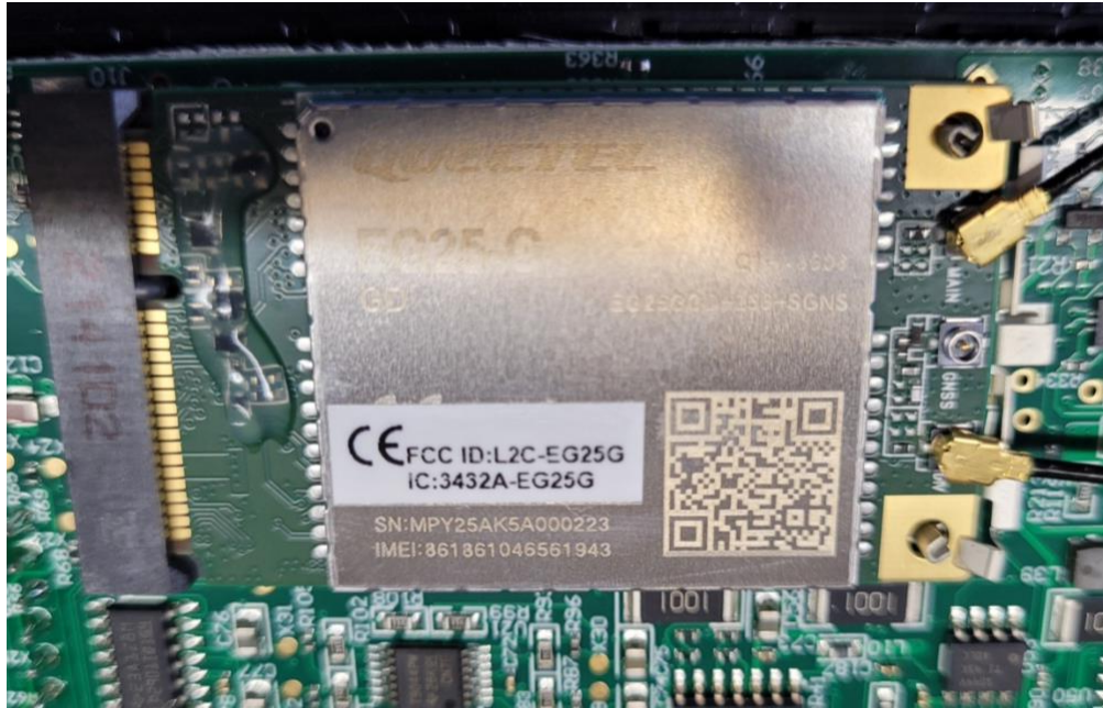
FCC/ISED Label on Quectel EG25-G Modem
