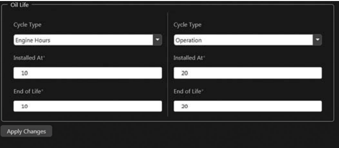
Figure 3-51. Oil Life Maintenance Setup
