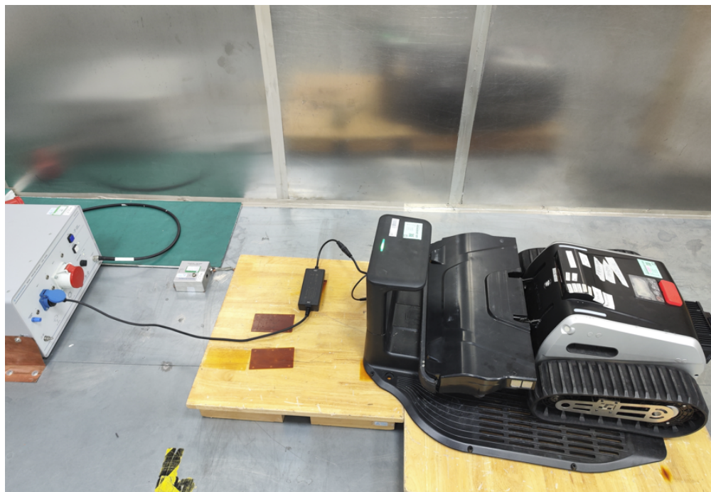
Photograph 3: Set-up photo for AC conducted emissions
