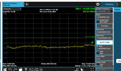
CH11 – 10th Harmonic of the fundamental frequency
