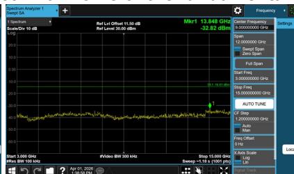
CH11 – 10th Harmonic of the fundamental frequency
