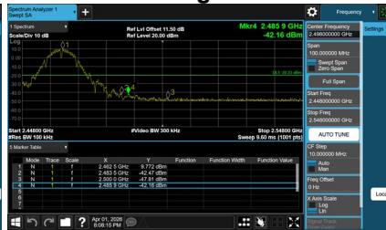
CH01 – 10th Harmonic of the fundamental frequency
