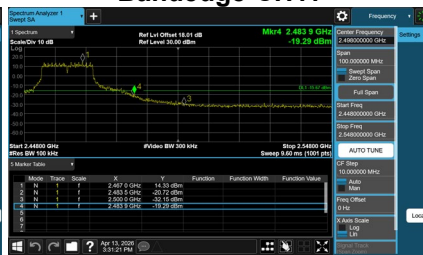
CH01 – 10th Harmonic of the fundamental frequency
