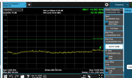
CH11 – 10th Harmonic of the fundamental frequency
