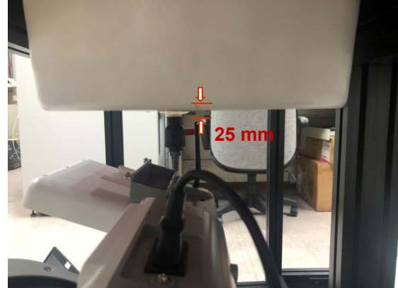
Photograph 2. Body, Top Edge of Antenna, 25mm
