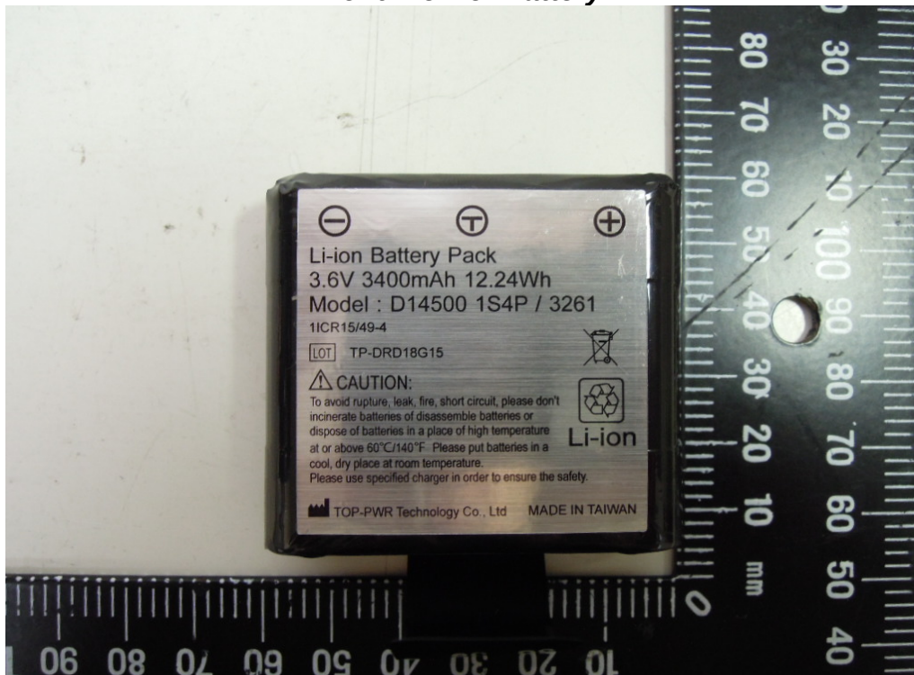
Front View of Battery
