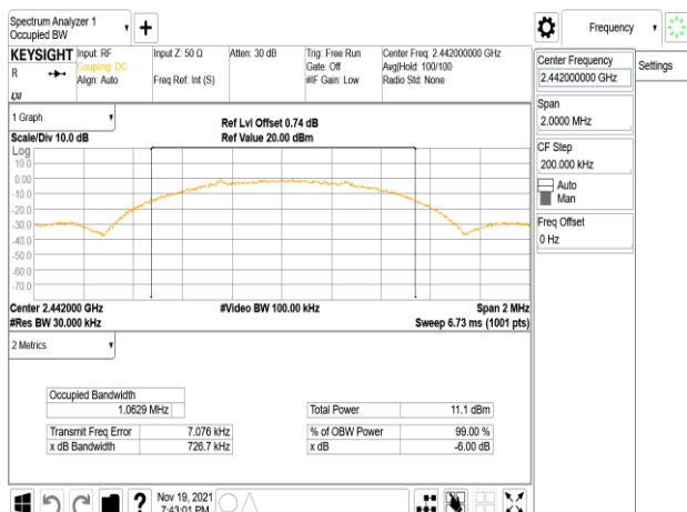
IC OBW_BLE 1M_HighCH39-2480MHz
