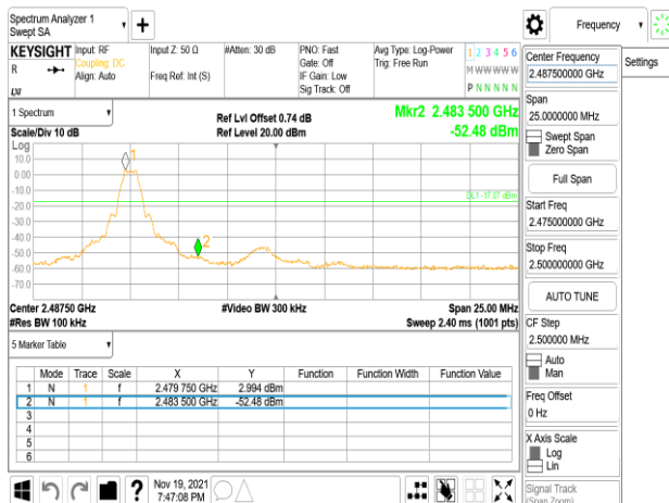
Band Edge_BLE 2M_LowCH00-2402MHz
