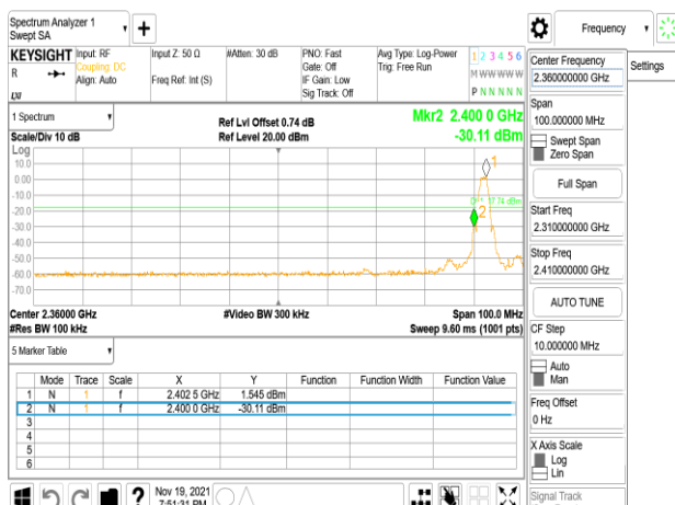
Band Edge_BLE 2M_LowCH00-2402MHz
