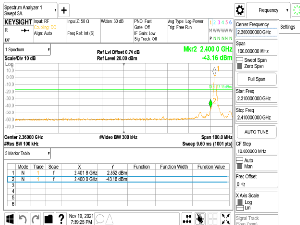
Band Edge_BLE 1M_HighCH39-2480MHz
