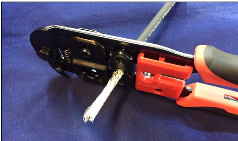
Figure 22: Crimping the Cable Strain
