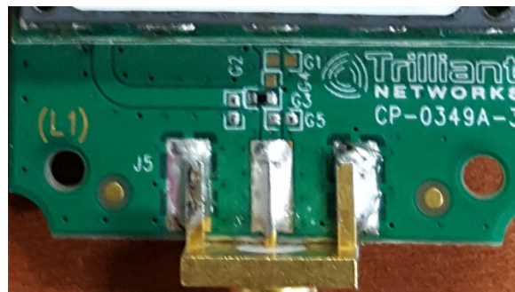
Figure 5 FCC and ISED approved trace design layout and picture for external antennas with SMA connector on side.
