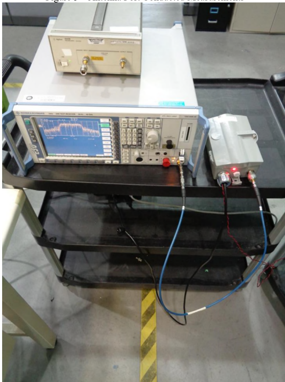
Figure 5 – Antenna Port Conducted Measurements
