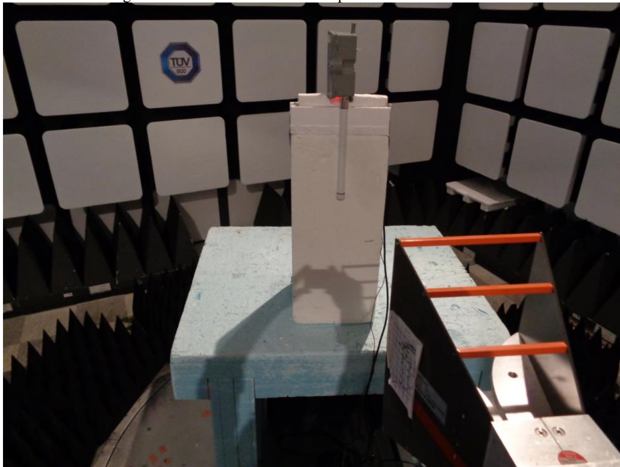
Figure 4 – Radiated Emissions Setup at 1m – 3 GHz to 18 GHz
