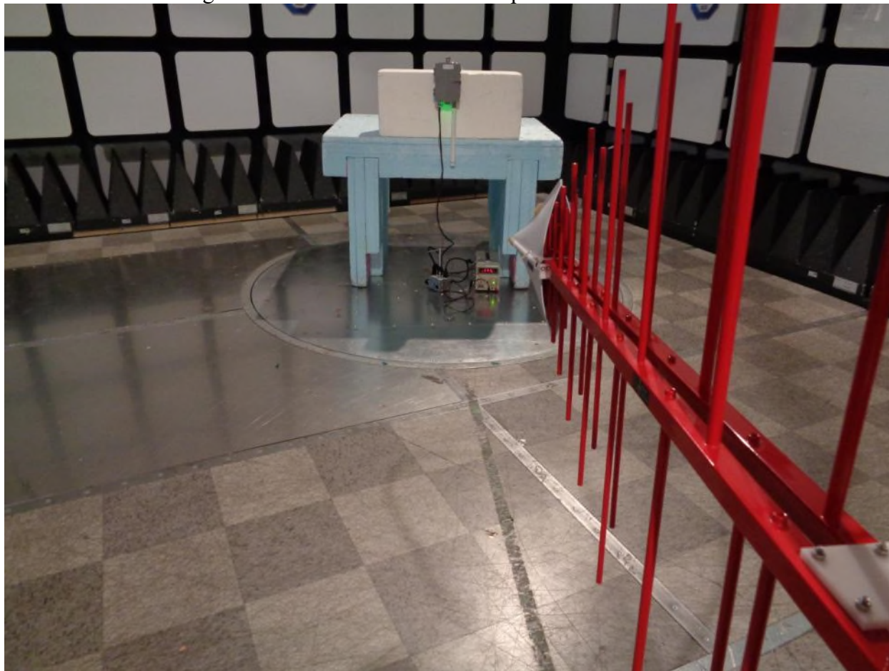
Figure 2 – Radiated Emissions Setup – 30 MHz to 1 GHz
