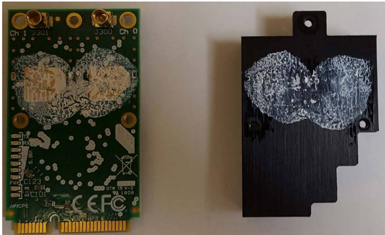
MikroTik radio bottom without shield
