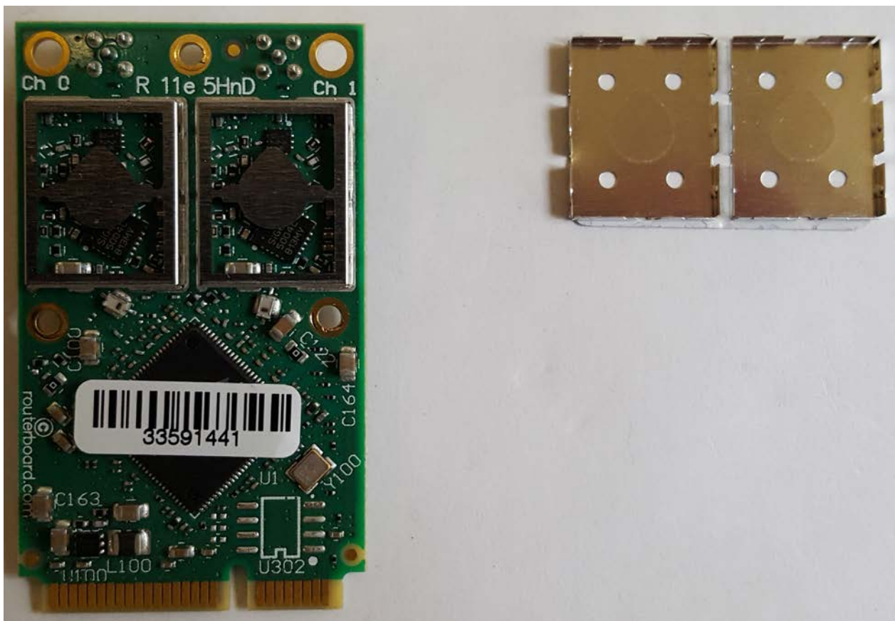
MikroTik radio bottom without shield
