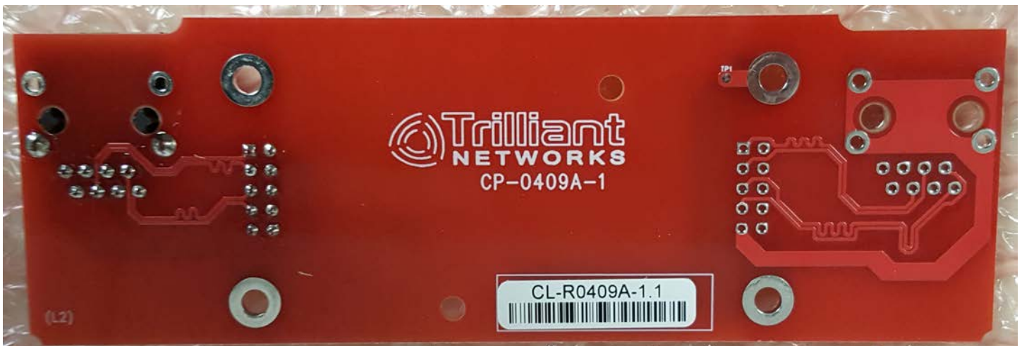
Ethernet I/O board bottom (PoE models)
