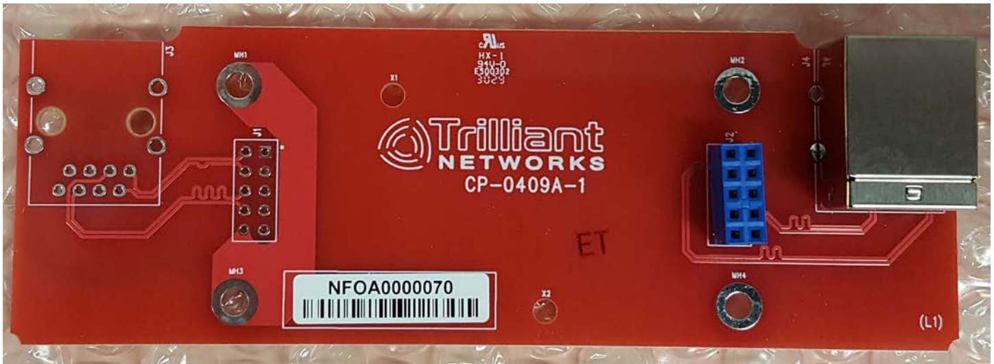
Ethernet I/O board bottom (PoE models)
