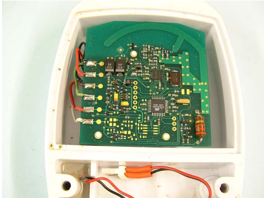
PHOTOGRAPH No.4 TRANSMITTER FRONT VIEW COVERS REMOVED
