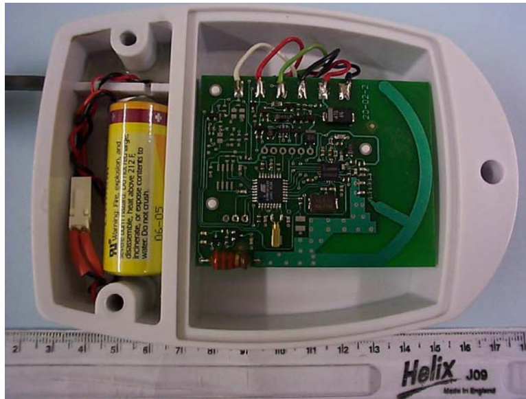
PHOTOGRAPH No. 2 TRANSMITTER FRONT VIEW COVERS REMOVED
