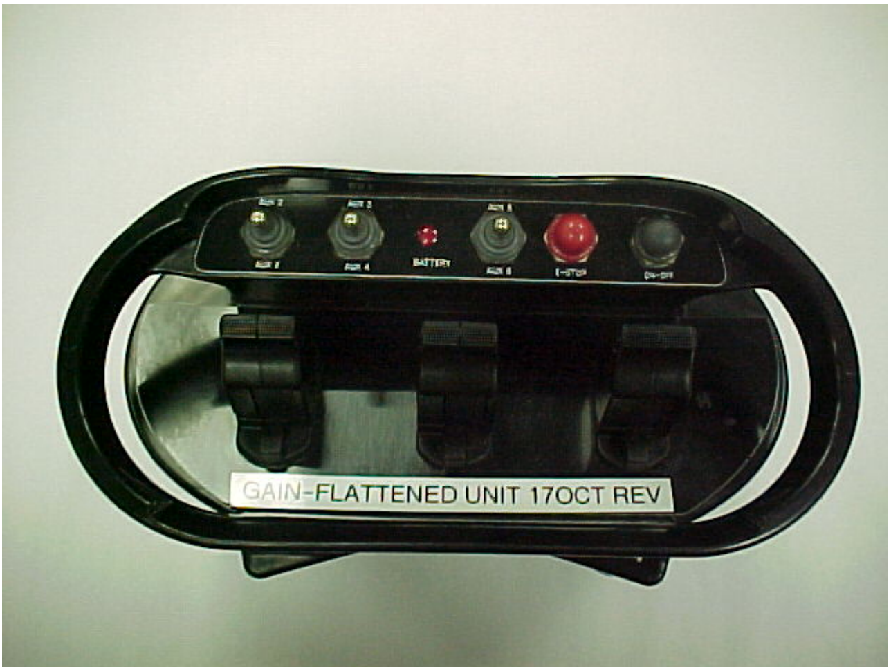
Photo Three – External Top View showing Control Switches
