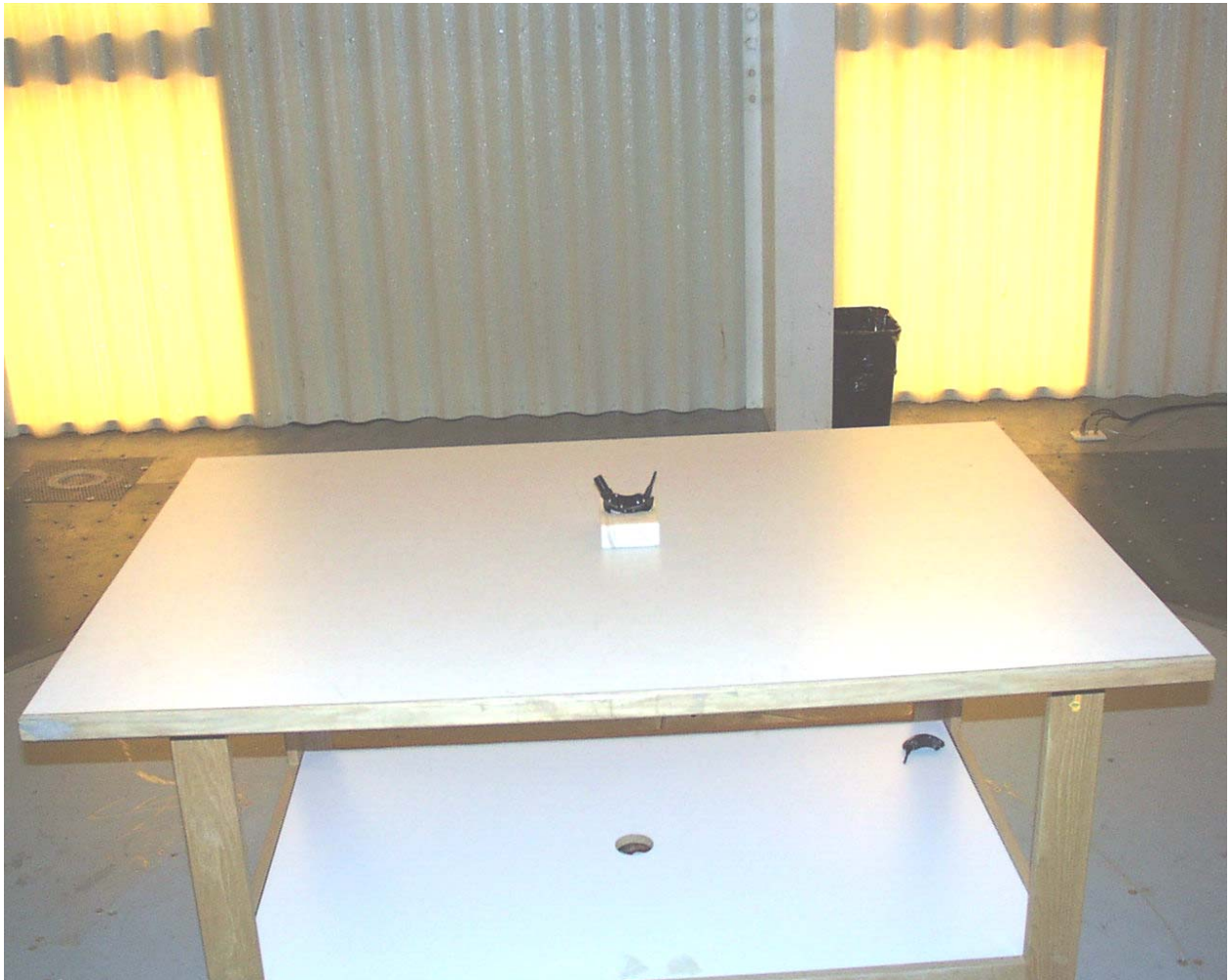
Front View of the Radiated Test Setup (Test Jig Configuration)
